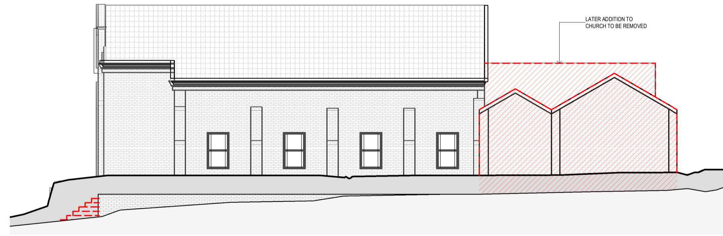
EXISTING + DEMO CHURCH EAST ELEVATION
