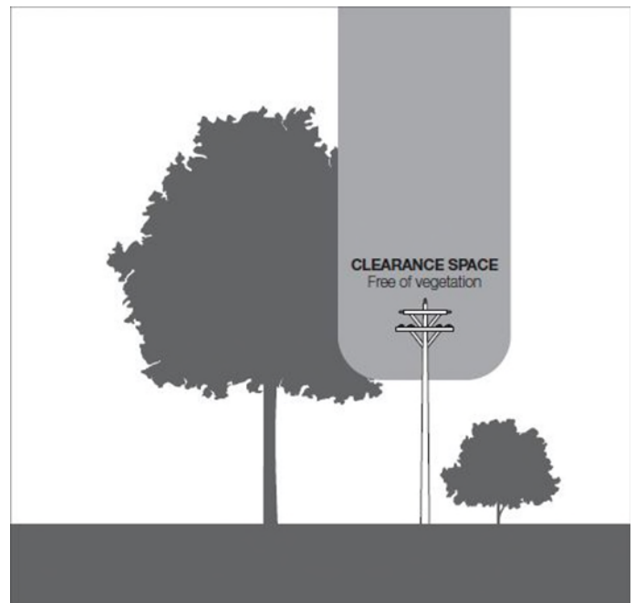
Figure 23 - Uninsulated 66 000 volt electric line in a low bushfire risk area and uninsulated electric line in a hazardous bushfire risk area (from ESELCR 2020)
