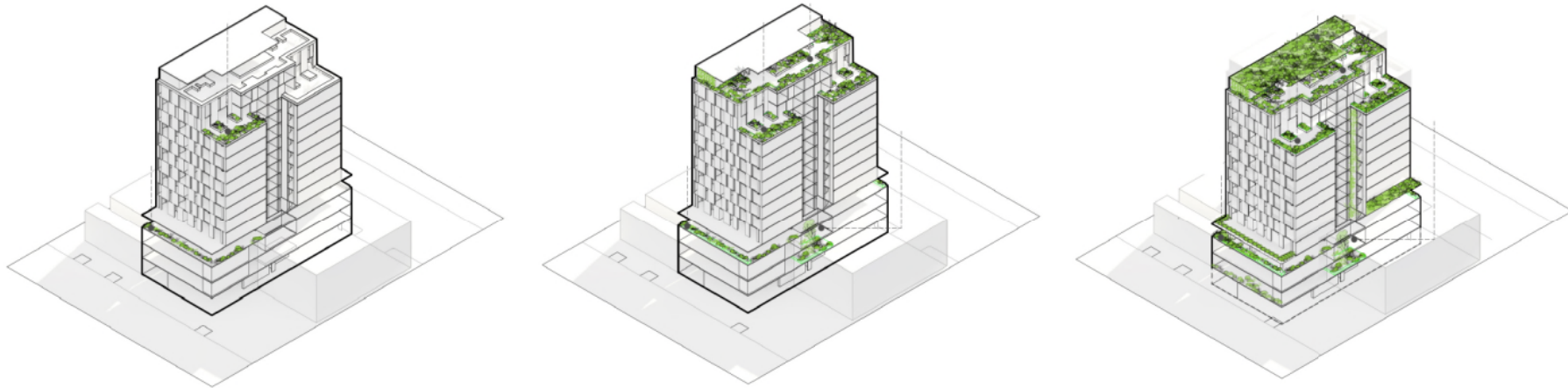
Greening scenarios for an example large residential typology. Business as usual scenario (left) showing a Green Factor score of 0.14, moderate greening scenario (centre) showing a Green Factor score of 0.55 and an optimised greening scenario (right) demonstrating a Green Factor score of 0.84. Images by SBLA
